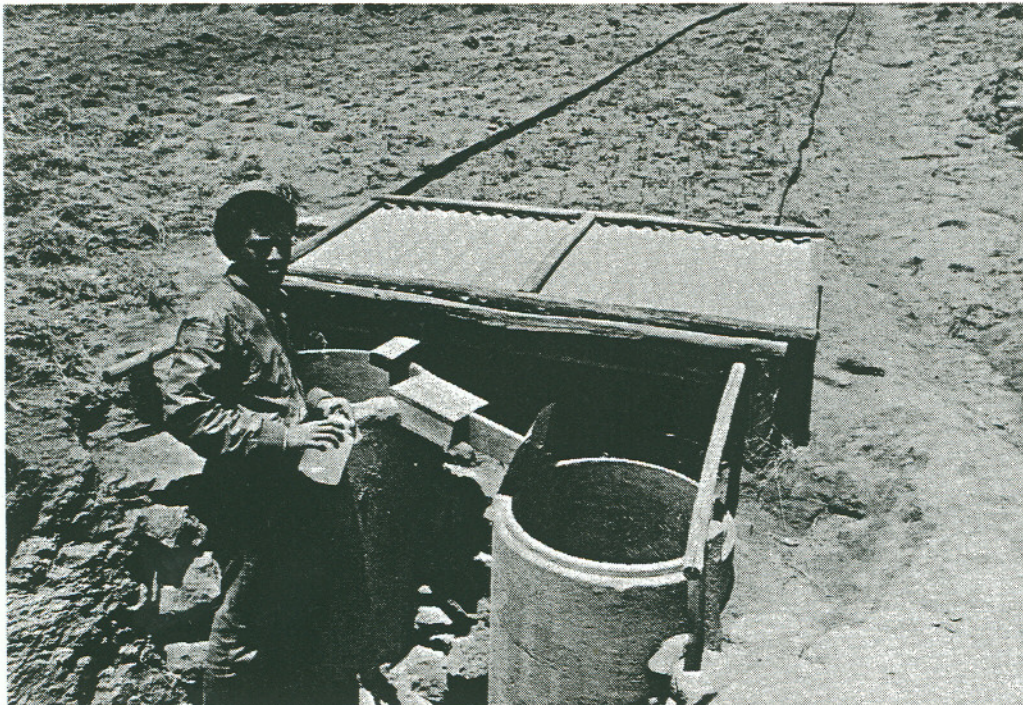
Testplot 1 at Andit Tid Station of SCRIP in the Hulet Wenz catchment set up to monitor runoff and soil loss as well as production on this traditionally managed field.
