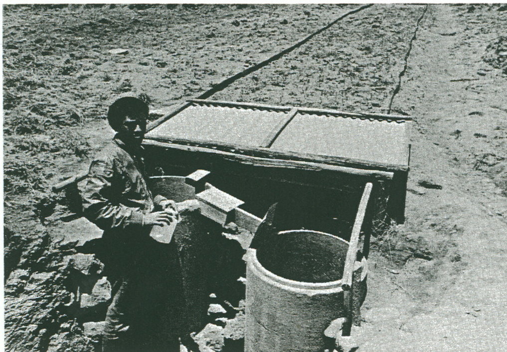
Testplot 1 at Andit Tid Station of SCRP in the Hulet Wenz catchment set up to monitor runoff and soil loss as well as production on this traditionally managed field.
