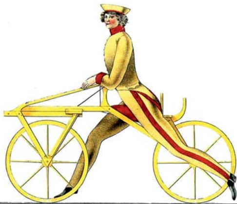
Fig. 24. Karl Drais’ walking machine (patent, 1817). The high prices for oat in the “Year Without a Summer” inspired Karl Drais to invent a “walking machine” without horses. This seemed to be a promising alternative in view of the increased costs for keeping and feeding horses. 216
