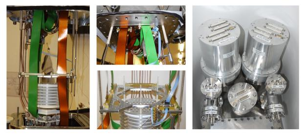
Figure 5.10: Photographs of the cabling of the TPC. Left, the cables of the charge-collection and light-collection system are guided to the top of the inner chamber. The brownish cables are made from Kapton. Middle down, the cables are fixed on the base plate with parts made from PAI. Middle top, the cables are fed through the bellow into the interface box. Right, view on the interface box with the electrical feedthroughs. The charge amplifiers are mounted directly on the feedthroughs.
