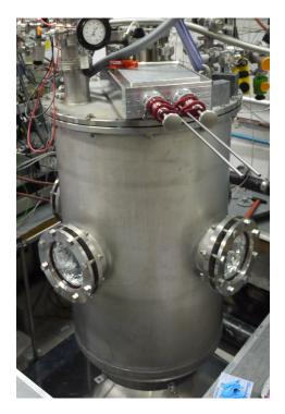
Figure 4.9: Photograph of the outer vacuum vessel. Through the view ports the supper insulation foil can be seen.
