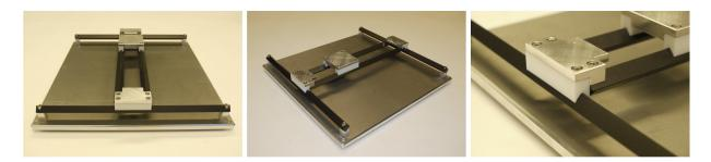
Figure C.3: Photographs of the current version of the displacement device. The rails are made from aluminium coated with Teflon.
