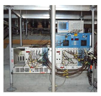
Figure 5.15: Photograph of the muon veto's electronic crates. The left crate contains the NIM modules of the muon trigger and the right crate contains those for the muon veto and the two PMT amplifiers. On top of it, the high voltage system and an oscilloscope for test purposes is placed.
