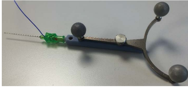
Figure 5: The needle equipped with a cable and a LED inside, attached to the adapter to connect the marker shield for the optical tracking of the needle.
