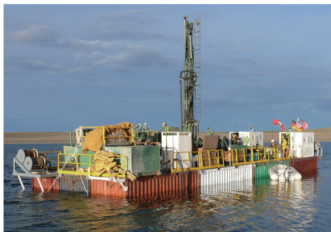
Figure 3. Platform R/V Kerry Kelts with the GLAD800 drilling system (center).
