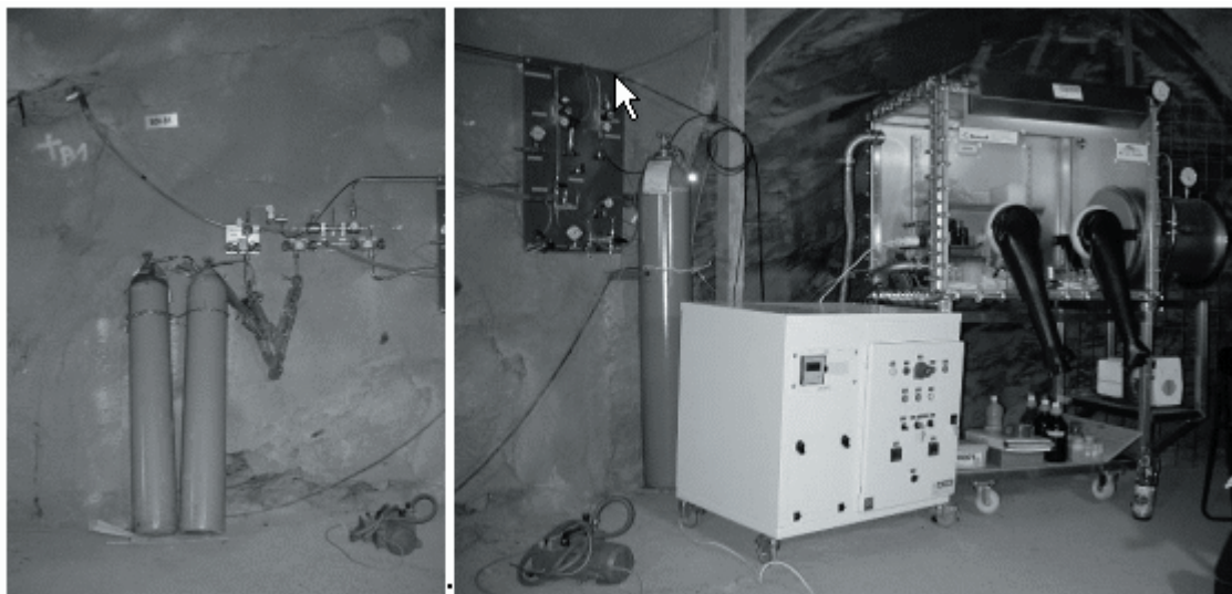
Fig. 9.- Surface instrumentation installed in borehole BDI-B1 for controlling the operation of the downhole equipment and for analysing and sampling in anoxic conditions.
