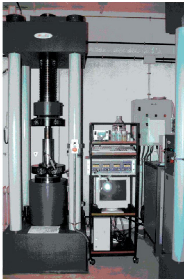
Fig. 10.- Photography and schematic representation of the pore water extraction device from core samples.
