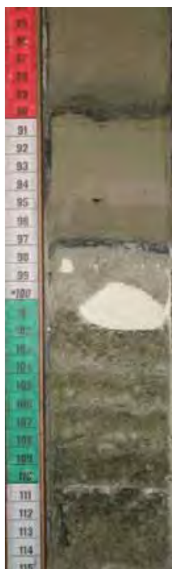
Figure 6. Sulfur nodule from ~99 to 101 cm in Core 6A-4H-2 near Pleistocene-Holocene boundary. Nodule formed near interface between underlying gypsum sand (Unit II) below and overlying clay (Unit I).
