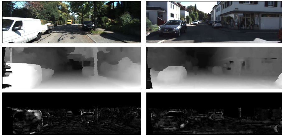
Fig. 8 Example results from the KITTI dataset. Top to bottom: left image, disparity map, and clamped disparity errors
