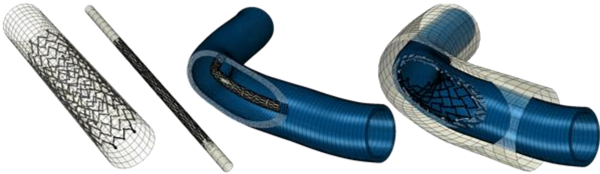
Figure 4.2. The preconditioning and deployment of a Nitinol stent into a patient-specific popliteal artery. By radially displacing the nodes of the expansion tool (not shown), the Astron-Pulsar stent is expanded to its unconstrained diameter of 7mm (left). After annealing, the stent is crimped to its deployment diameter of 1.2 mm by radial displacement of the nodes of the crimp tool (middle-left). The insertion to the patient's artery is achieved by a displacement-controlled deformation of the crimp tool into the shape of the arterial midline (middle-right). The crimp-tool is then expanded to its initial diameter, which corresponds to the deployment of the stent as it is detached from the tool to contact the arterial walls (right).
