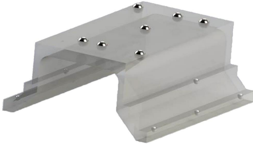
Figure 3.1. The phantom that is attached to the patients' legs during image acquisition is used to calibrate the 2D angiographic images using the fiducials embedded into its surface.
