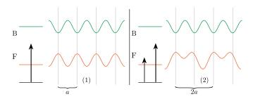
**Figure 2.** Realization of the staggered lattice structure. The black arrows indicate the dipole lasers which are used in the experimental setup. (1) Blue/red detuning for fermions/bosons generates phase-shifted optical potentials for bosons and fermions with a lattice period *a*. (2) The superposition of the lattice with period *a* by a superlattice of period 2*a* generates the staggered structure for the fermions.
