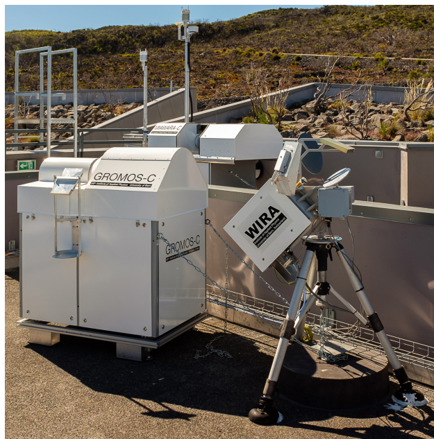
Figure 1. The ozone radiometer GROMOS-C at the Maïdo observatory, on Réunion island, together with the wind radiometer WIRA and the water vapour radiometer MIAWARA-C.
