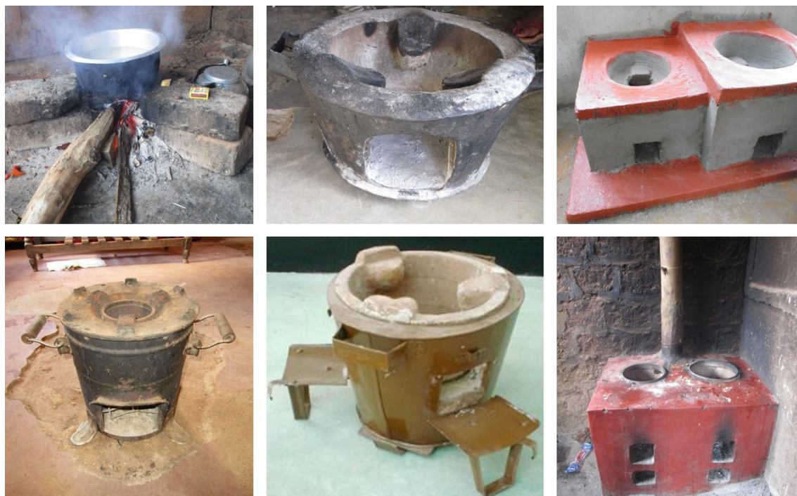
Photo 1. Firewood stoves. Top (from left to right): three-stone fireplace, Maendeleo, Rocket ; bottom (from left to right): Envirofit, Kuni Chache, and Okoa .
