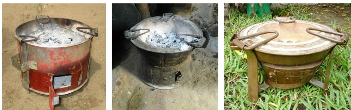
Photo 2. From left to right: unimproved charcoal stove, Kenya Ceramic Jiko (KCJ), and Sazawa charcoal stove.
